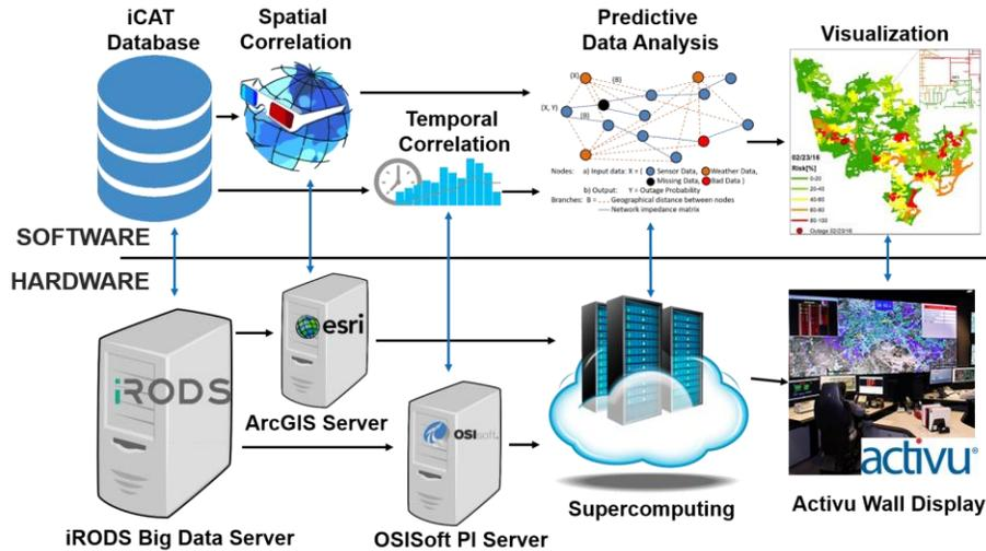
Figure 1. Weather testbed architecture.
